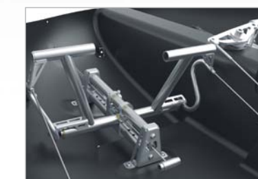
Individually adjustable: pedals can easily be adapted to the pilot's size.
